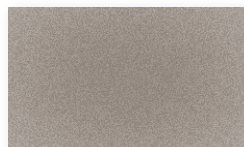
Weathered Galvalume SR=.34 E=.82 SRI=34
